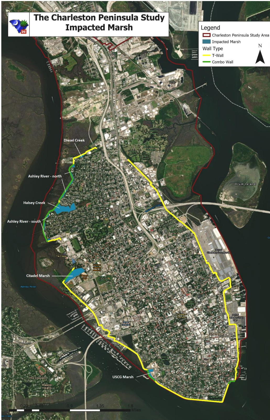
Figure 8. Map showing areas of salt marsh (estuarine emergent marsh) potentially affected by the storm surge wall where it would be constructed in the marsh.
