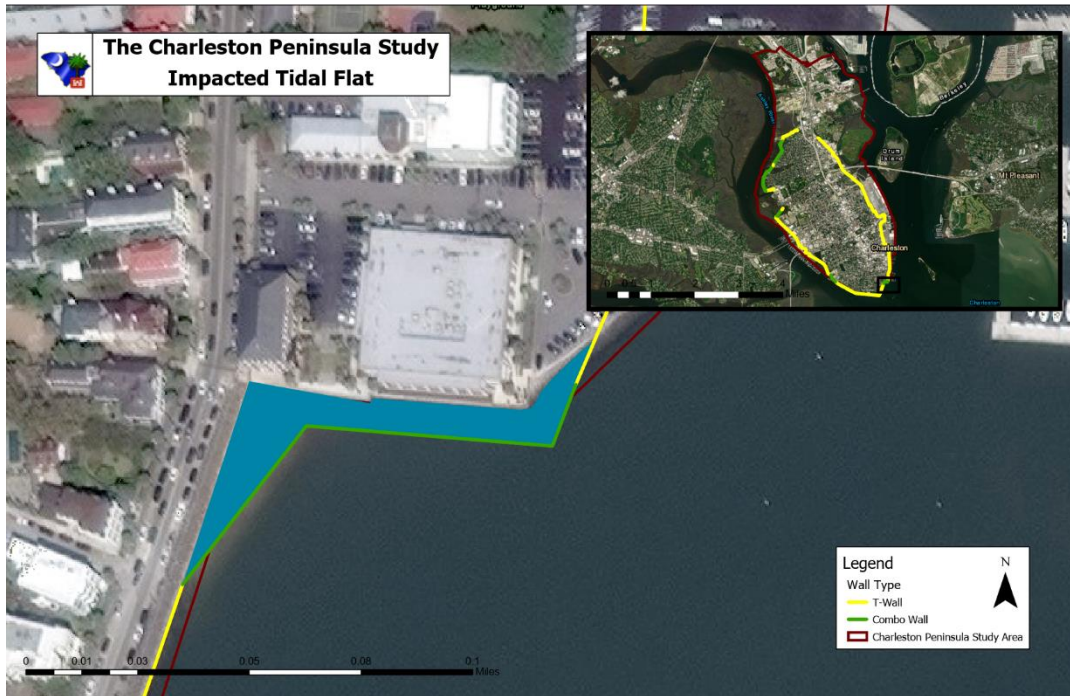
Figure 11. Location of intertidal sand flat (shaded in blue) that would be affected by the proposed storm surge wall at the northern end of the High Battery Seawall.
