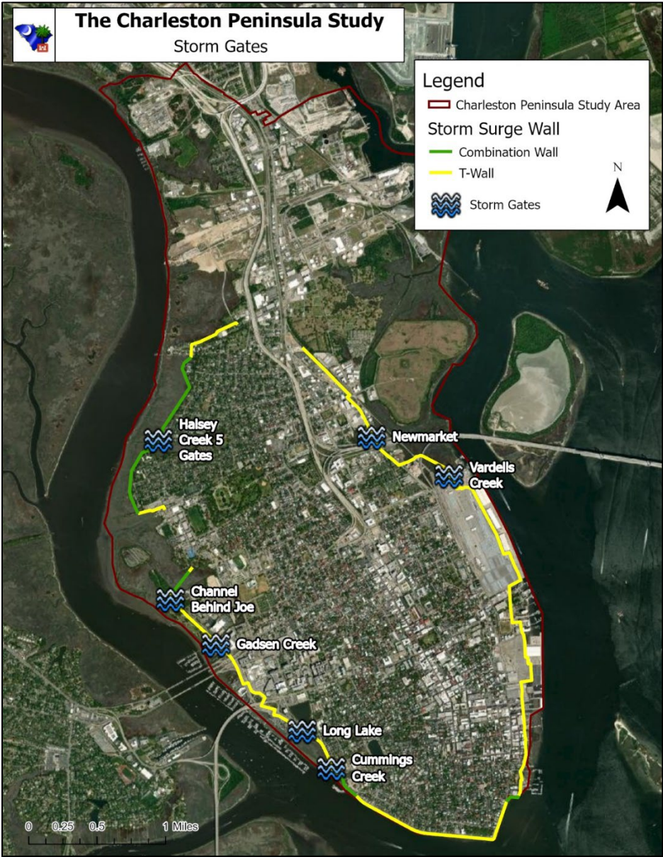
Figure 7. Planned locations for storm gates; six of the gates are under roads that intersect the creeks/channels.
