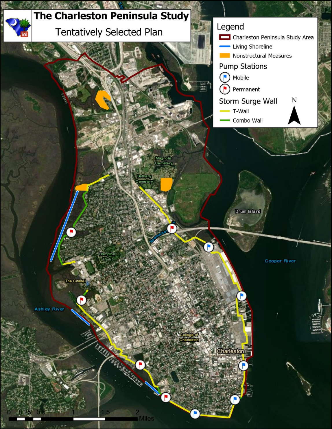
Figure 2. Map showing the measures and some of the features of the Tentatively Selected Plan.
